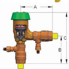
The Apollo Model PVB 4A or PVBLF 4A Pressure Vacuum Breakers are designed to prevent contamination of potable water due to back-siphonage. An integral relief valve serves to reduce the possibility of damage due to intermittent freezing conditions. The modular check valve cartridge has a replaceable seat and a reversible silicone seat disc. Ball valves with stainless steel handles and nuts are standard.
