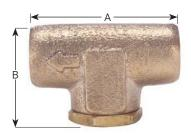
The body of the 59-V is corrosion-resistant solid cast bronze, ASTM B-584. The removable clean-out cap is solid brass, ASTM B-16. Standard screens are made of 304 stainless steel. NOT INTENDED FOR POTABLE WATER
