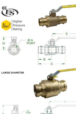
The APOLLOPRESS® 77V Series two-piece press ball valve is ideal for installation in most HVAC systems. Features Leak Before Press® technology and 300 psig maximum working pressure. Proudly Made in the USA.
