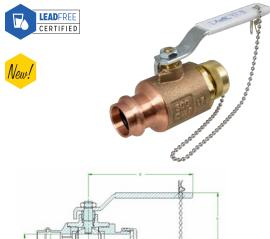
Designed for direct mechanical connection to ASTM B88-Type K, L, and M copper tubing in the hard drawn condition for sizes 1/2"-3/4". Valves feature a 3/4" hose thread connection with heavy brass cap to protect the threads and is full pressure rated. Features copper retainers for maximum protection against corrosion and dezincification. Not for use with natural gas.
