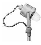
2" tapered threads (2 - 11-1/2 NPT). Locking Screw for horizontal adjustment. 30" Flexible Coupling connects to 3/4" fixture hub (3/4 - 14 NPT) and to 1/2" pole-top opening (1/2-14 NPT).
