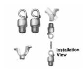
Complete assembly includes two hooks and one rigid support. Each hook supplied with a screw for closing 3/8" jaw opening. Rigid Support straddles max. 1-1/4" conduit. (Chain shown in installation view not furnished.)
