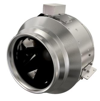
The housing is manufactured from a two-piece stamped, galvanized construction. The fan motor can operate in temperatures of air up to 104°F and the motor bearings are permanently sealed and self-lubricating for maintenance-free life.
