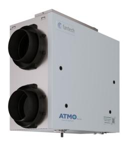
The appliance features an efficient crossflow heat exchanger with SRE up to 75%, standard MERV3 filters, a drain hose and hanging chain kit <sup>1</sup>, easy connect ports, integrated air balancing taps and duct ports with plastic collar shrouds for simple and quick installation. Comes with a limited warranty (lifetime warranty on the exchanger, 7 years on motors and 5 years on parts).
