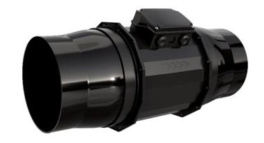
With the motor in the airstream, the fan provides the constant dissipation of heat build-up even at partial load that gives this fan best-in-class longevity and reliability backed by an industry leading warranty. For the same air volume, the prio**AIR** EC fan consumes considerably less energy and pushes up to 50% more air than a non-prio**AIR** AC fan of its size. Additionally, the optimized shape of the aerodynamic optimized impeller provides an ideal air stream.
