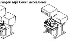
Sample Assembly Drawing for Finger Guard Installation (for 150VA to 1500VA)
