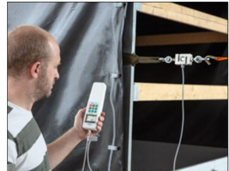
Universal digital force gauge for tensile and compressive force measurements with external load cell
