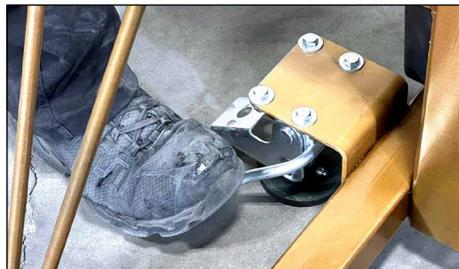
11. To remove pail from holder release web strap and open can holder.
