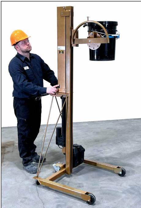
6. Press toggle switch on mast upward to raise pail to pouring height.
