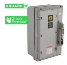
Safety switch, heavy duty, non fusible, 30A, 3 poles, 30hp, 600VAC/DC, NEMA 4X krydonTM fiberglass polyester
