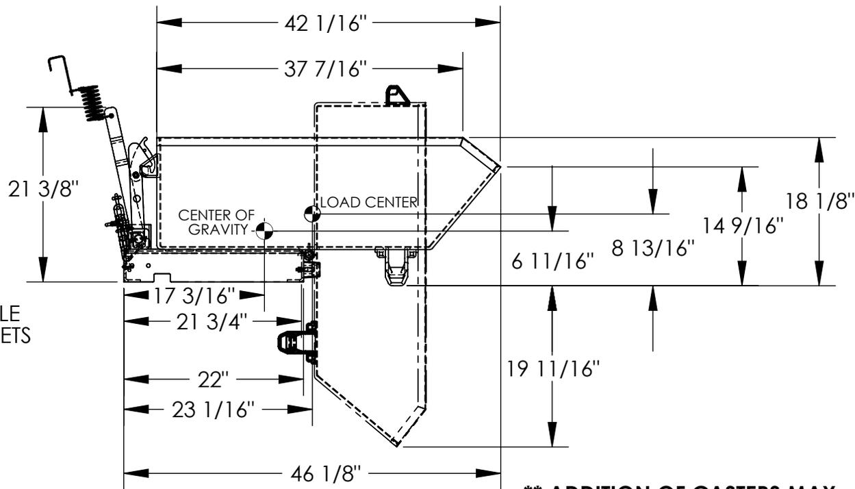
NEVER EXCEED LOAD CENTER RATING PER FORK TRUCK MANUFACTURER'S GUIDELINES. DO NOT USE THIS FORK TRUCK ATTACHMENT IF LOAD WILL EXCEED FORK TRUCK MANUFACTURER'S LOAD CENTER RATING.
